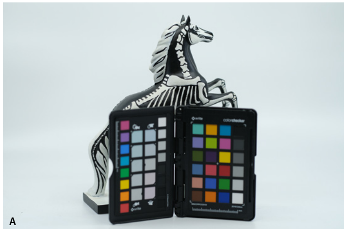
Fig. 1: AF-S Focus Priority (A) vs. the 'improved' version of AF-S Release Priority (B). In this test, I autofocused starting at the minimum focus distance of the XF90mmF2 lens and fully pressed the shutter button. In AF-S Focus Priority mode (A), the camera and lens take the time they need to finish and confirm the focus run when the shutter button is fully pressed. With the new version of AF-S Release Priority mode (B), pressing the shutter button stops the autofocus in its tracks and the camera immediately takes the shot, whether or not it is in focus. In this case, it clearly is not.
